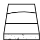
24" MIDDLE/BASE HALF BLOCK (MAY BE CAST w/o TONGUE TO AVOID FIELD CUTTING)
