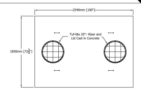
WORKING VOLUME to liquid depth: 4800L (1050 GAL) TOTAL VOLUME to underside of lid: 5700L (1250 GAL)
