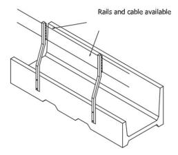
Increase your overall efficiency with a fence line feed bunk system. At Boyd Bros, we use modular designs that conform to your site requirements, and are made from high strength 50MPa, air-entrained concrete with heavy steel reinforcing; ensuring unsurpassed safety and durability. Feed bunks can be placed in a field on existing soils, in a barn or even on a concrete pad- We can work within your guidelines to make you exactly what you need.
