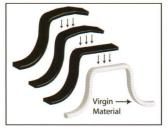
Our multi-layered tank construction, consisting of virgin material surrounded by 3 layers of protection.
