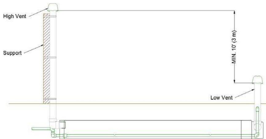
Figure 47. Differential venting – Low-pressure Distribution for Standard Configuration
