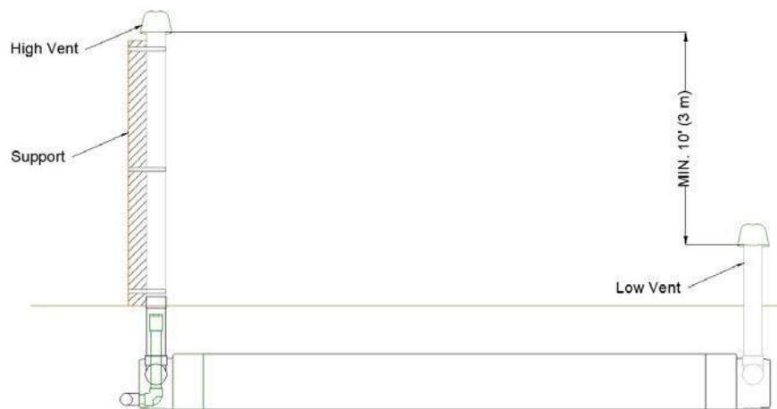
Figure 47. Differential venting – Low-pressure Distribution for Standard Configuration
