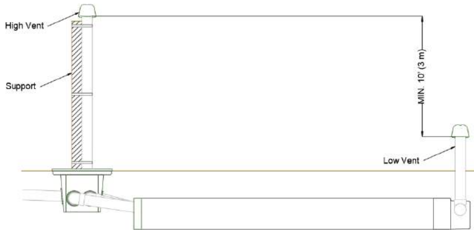
Figure 46. Differential venting – Standard configuration
